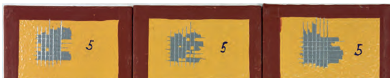
Fig. 4 Cross-cut test of coated steel panels after 720 hours of NSST; panel width is 100 mm
