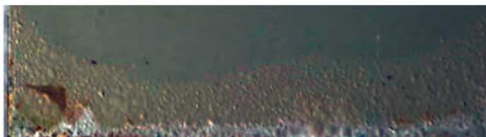
Fig. 1: Large delamination from cut edge of coil coated steel panel after 12 weeks of a cyclic corrosion test; the panel width is 100 mm
