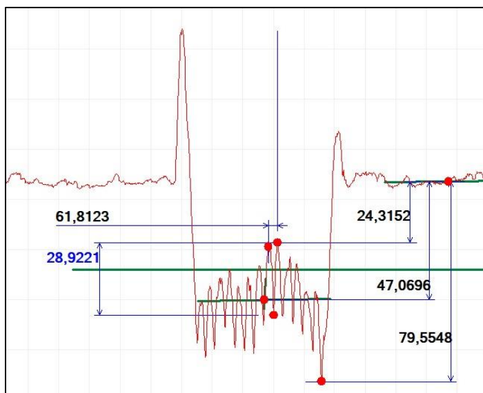
Figure 8: Example of evaluating the depth of structuring on a steel substrate using SurfTest SJ 500P roughness tester software
