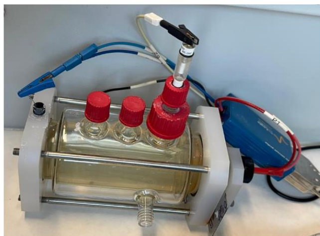
Figure 9. Experimental set up for linear polarization test
