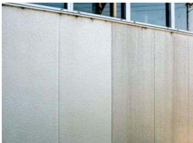
Fig.4: Comparison of self- cleaning paint (left) and conventional paint (right) in atmospheric conditions
