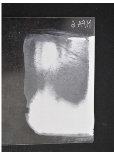
Fig.3: Degradation of organic binder during weathering in QUV panel
